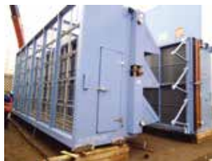
Turbine Inlet Air Heating System For Anti-icing
